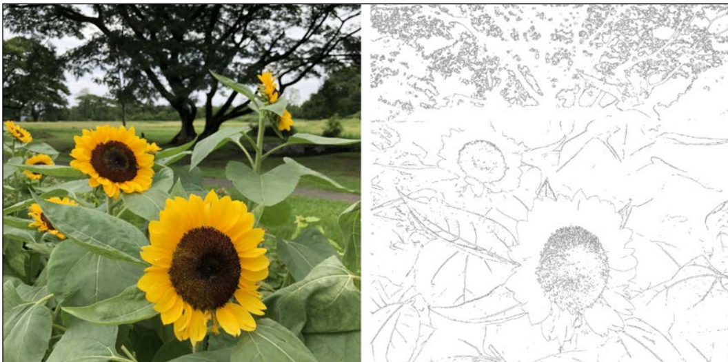
Figure 7.1.1: Example of an aligned image pair: left, original image, and right, transformed image using a Canny edge detector. The original photo was taken by the author.
