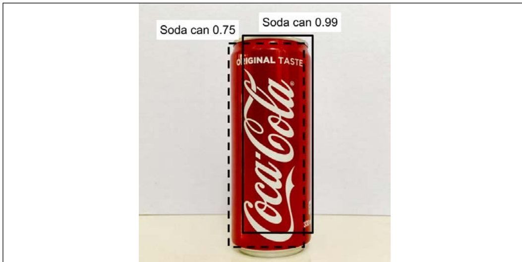
Figure 11.12.1 The network predicted two overlapping bounding boxes for the Soda can object. Only one valid bounding box is chosen and that is the one with the higher score of 0.99.
